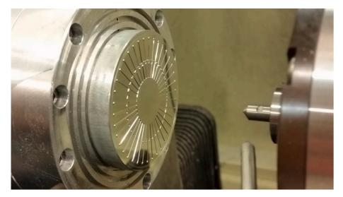
Manufacture of a molding tool for the production of blood plasma separators based on micro-fluid principles with a minimal structural dimension of 15  $\mu$ m
