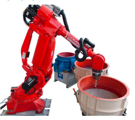
are available in the institute's test field as well as a centrifugal disc finishing machine. A 6-axis robot NJ 370, Comau Robotics, is used for workpiece guidance in drag finishing processes.
