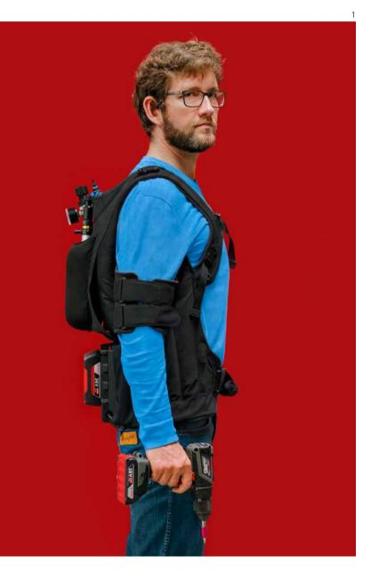
The exosuit contains almost no rigid elements. Instead, force relief is provided via precisely applied compressed air.
