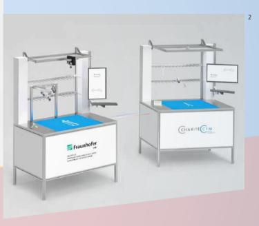
of an automated training process. The overall system is implemented in accordance with the two-man rule as a supplementary testing instance for employees in the packing process and aims to help document the work steps on the packing trays as well as ensure their quality. This aims to reduce the number of complaints regarding incorrectly packed trays.
