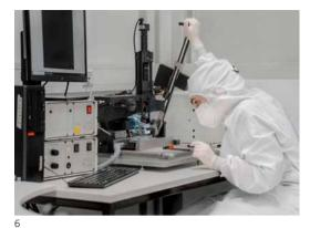
In the ISO Class 7 **cleanroom** which complies with DIN EN ISO 14644-1 (image 8), research teams develop coating strategies and production technology-based scaling methods for micro- and macrofluidic systems in a controlled atmosphere. Prototypes and small series are also manufactured here at the request of customers.
