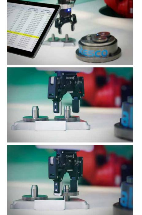
Images: Complex automated assembly processes can be piloted more costeffectively in the future with the help of digital twins. A single modular development environment serves as 15 assembly stations.
