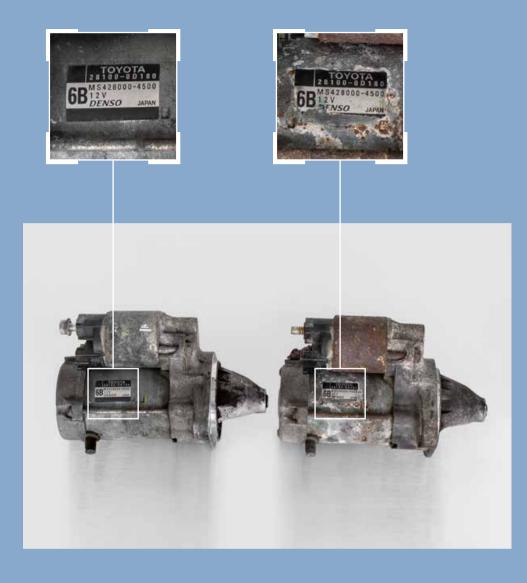
Image: Condition variance – two starters with identical part number differ visually due to signs of wear.
