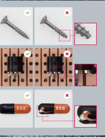
Images: Detection of defective screws transistors and encapsulations © MVTec Software GmbH
