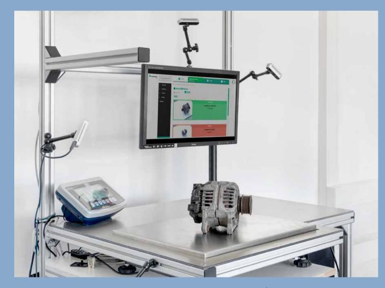
Image: Al-supported decision support system for semi-automated sorting of used components
