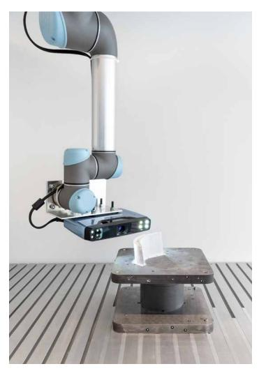
With Scangineering, CAD models can be automatically derived from 3D scans of objects.
